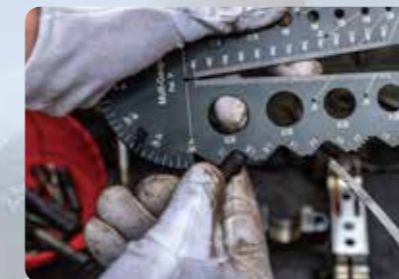
Pitch Size Measure the Thread
