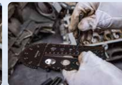
Gage Holes Select Right Size Drills
