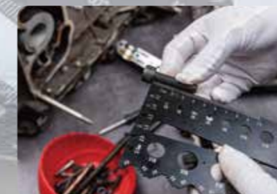
Gage Leg Quick-Check Perpendicularity
